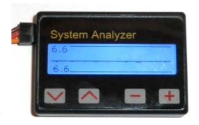
New test with same battery (LiFe 6.6V) but with a servo connected and loaded with a 2Kg weight. There are voltage variations due at servo "buzz", but of a value about 0,05 V, voltage never goes close to 6,5V.
