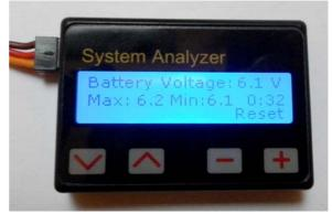
maximum and minimum voltages read from battery. If there has been a glitch to the power that caused the system to reset, the time counter reflects the actual period analyzed that maybe shorter than full flight.
