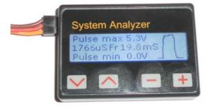
It is possible to test the signal quality at several places (after receiver, after the battery splitter system, on long leads...But it is recommended to do the test with all devices connected, if you want to measure the signal quality that arrive to a servo, you should use a "Y" lead and "look" at the signal with the servo connected, to take in to account the influence of the servo itself.
