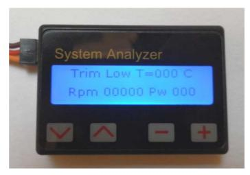
mode to battery analyzer mode, press on the (-) button during 10 seconds. Refer to System Analyzer section for a description of the functions.
