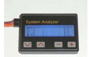
Trough the buttons + and - it is possible to modify the speed of the displayed data, making possible to analyze in detail slower or faster events.
