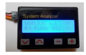
First screen displayed is the measure of the principal parameters, battery voltage and pulse width.
