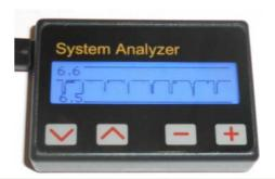
Same test and load, but in this case using an old and tired NiCd battery. Voltage variations are of about 0,3V, 6 times more than previous test. Voltage drops momentarily to 4,6V under load. A measure with a standard voltmeter would show the average voltage wich would be around 4,9V.
