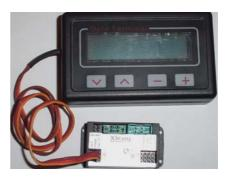
Connect the RPM sensor and thermocouple on its respective sockets, in the orientation that is shown in the colored labels on the fadec. If necessary, both leads can be extended using good quality servo extensions.
