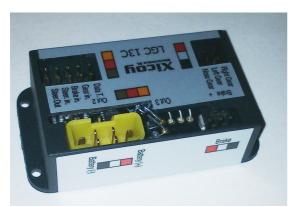
Connect the leads from brakes on the sockets labeled "Brake". Polarity and position are not important on the brakes.
