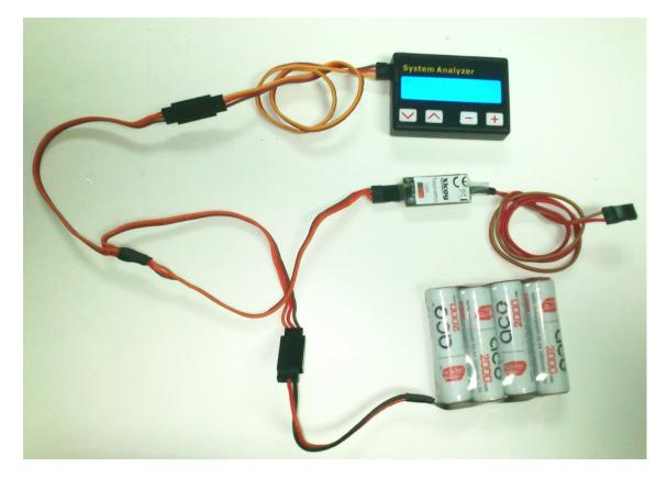
The RED led on the adapter will lit, and the data terminal will display "Radio Model: JETI" when new from factory. Through the "+" button you can change to another supported brand.
