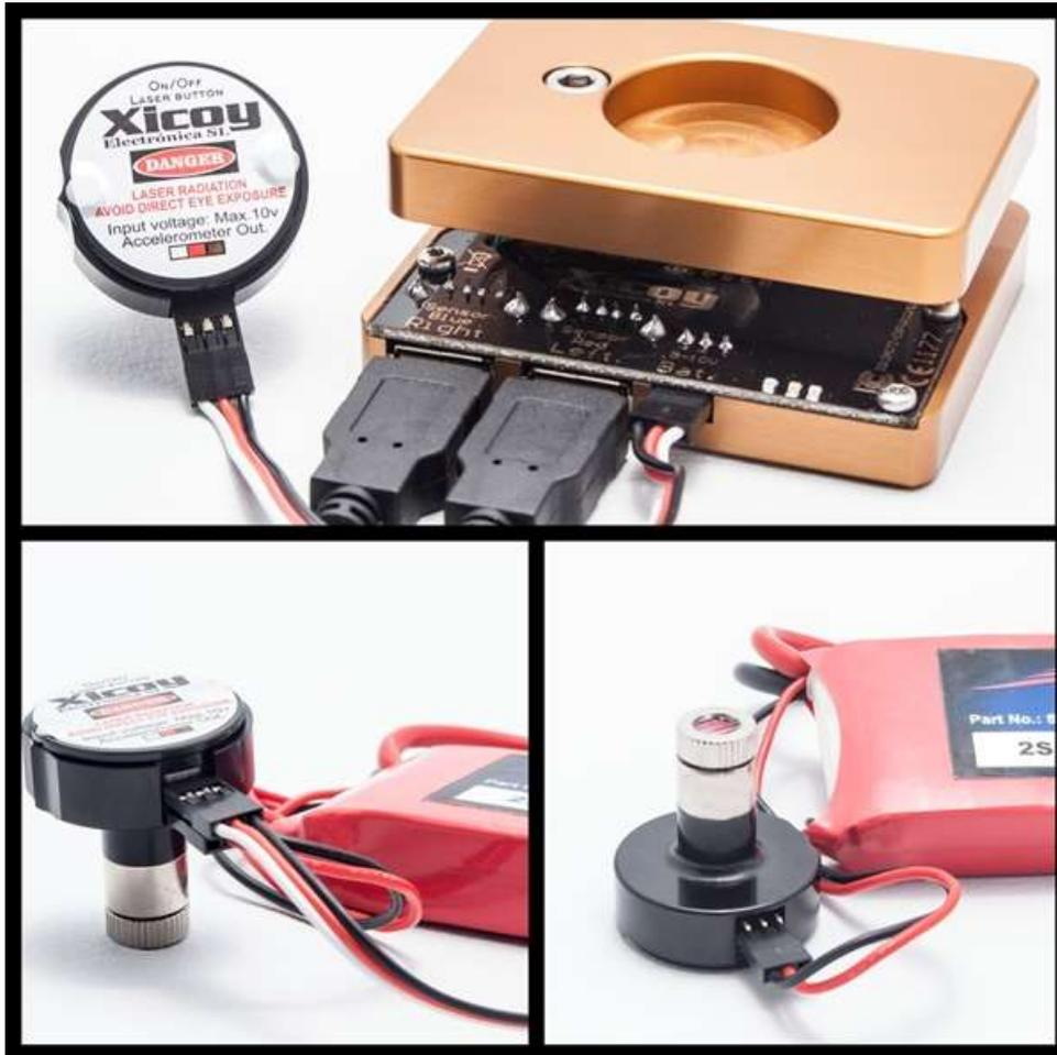
If you own the laser module, it includes an angle meter to be used to measure and adjust the deflection angles of the surfaces.
