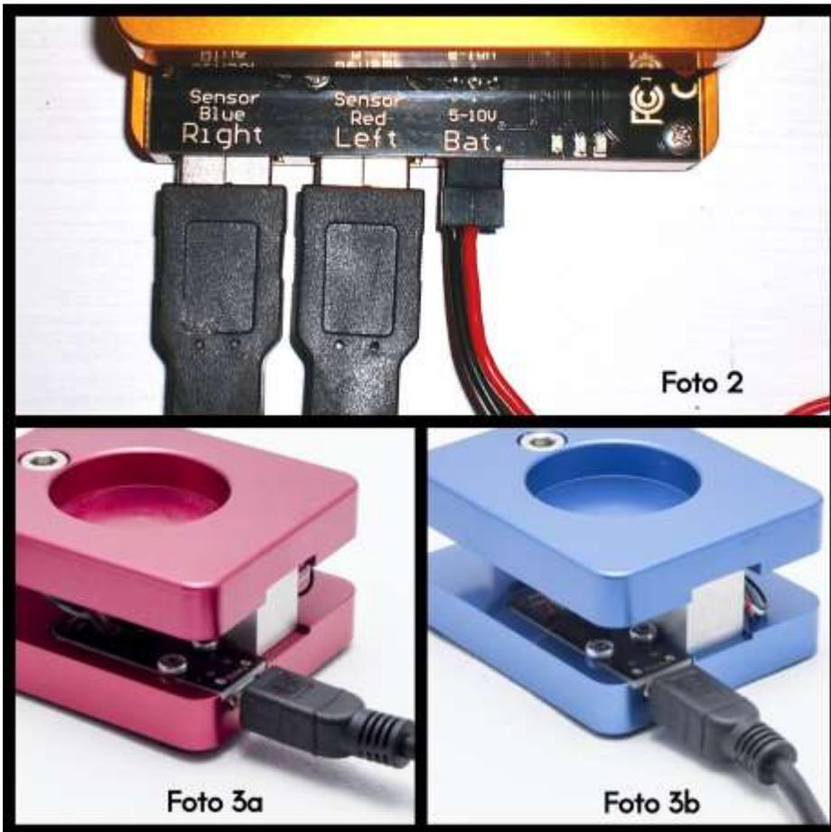
Connect the Blue and Red sensors to the yellow main unit using the leads supplied each sensor in its own socket. Connect a battery between 5 and 10 volt on the battery socket as per **picture 3a 3b**.
